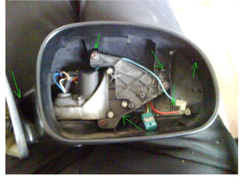
Undo the 6 torx 20 screws (green arrows) and lift out the black bit of plasic, now remove the wing mirror covering
