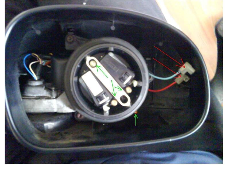
Undo the 6 clips that hold on the backing plate (green arrows) try not to snap them
