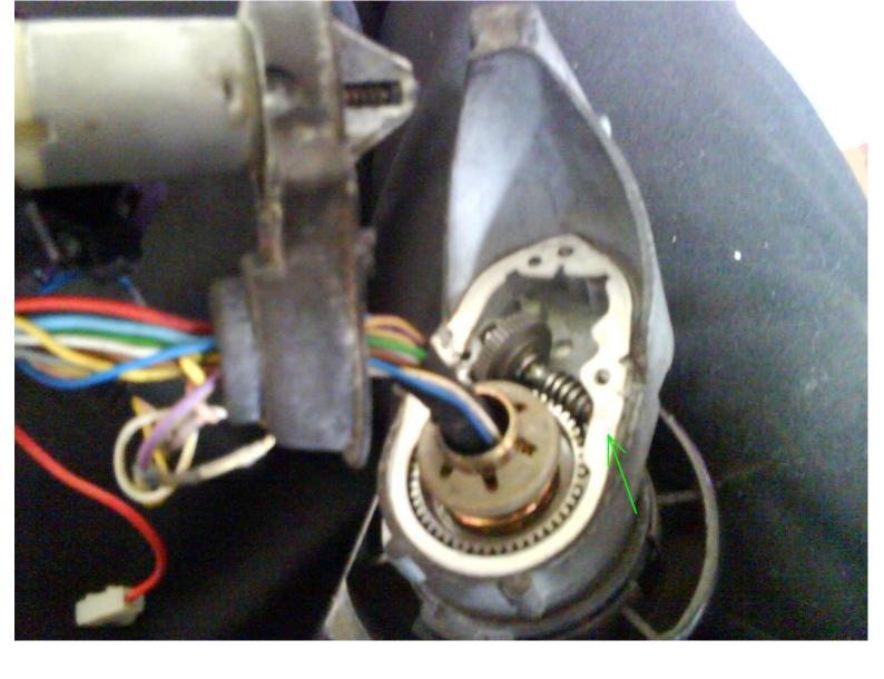
Take note of the worm gear shaft has 2 copper runners with 2 small metal bearings:
