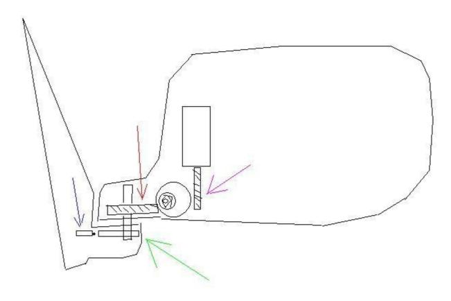
Manual fold point screwed on to the mirror base plates (green arrow)
