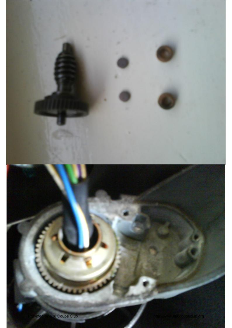
Now here mine was rock solid could not turn the gear at all, after alot of strenth and trying I finaly got it to losen up
