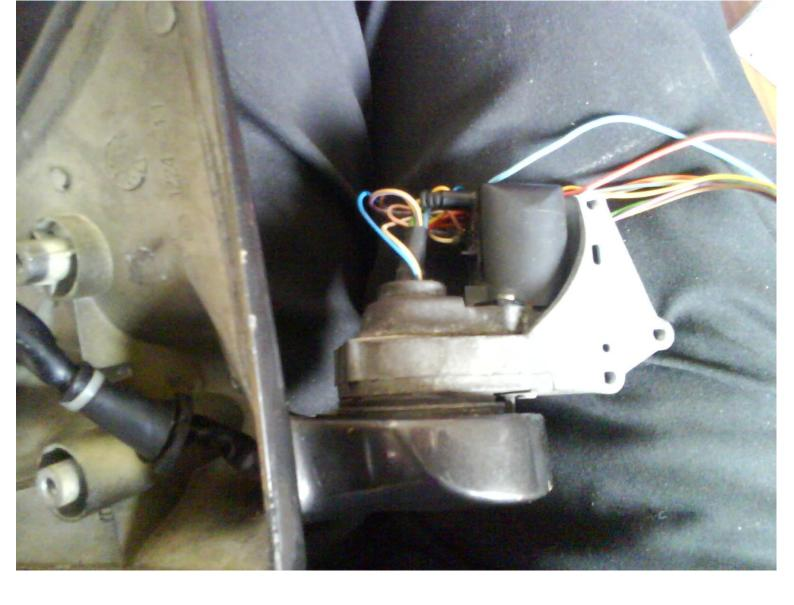
Now pull back the rubber grommet on the motor cover:
