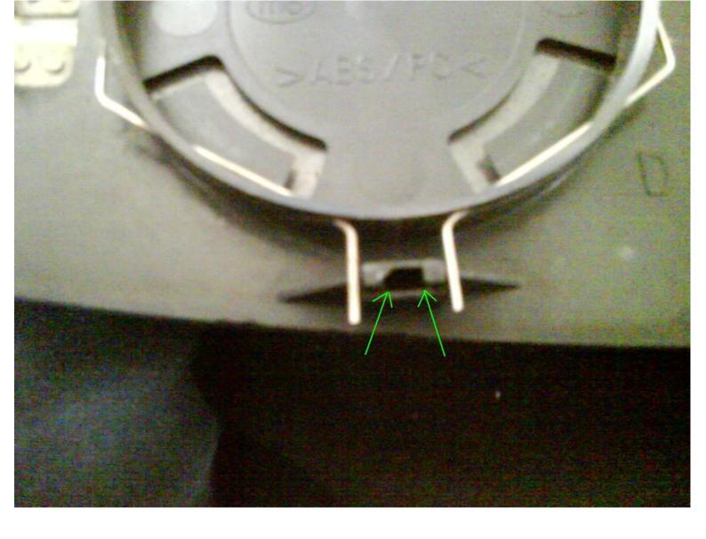
Once this is down lift out the mirror and undo the heated glass connections (red arrows) now undo the 3 torx 10 screws (green arrows) and lift out the motors and undo the blue connector
